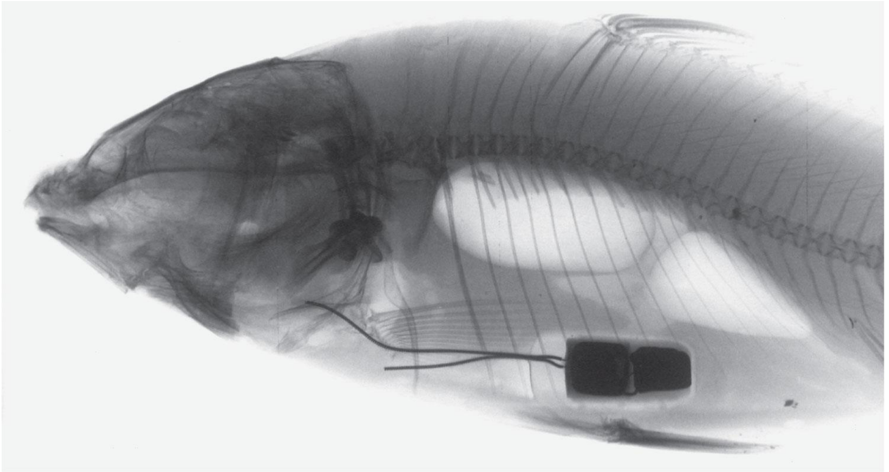
(c) Goldfish with implanted sensor for ECG
